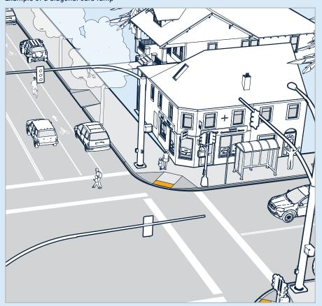
Example of a perpendicular curb ramp
