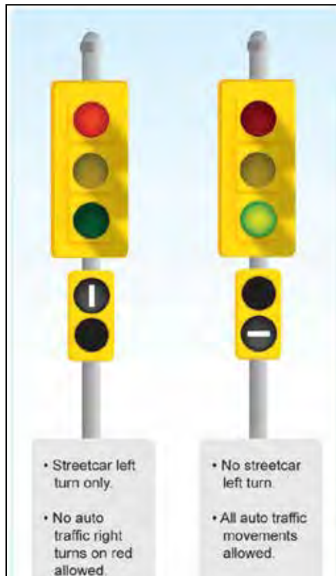
Figure 35: Example of a Transit Signal Phase for Streetcar
