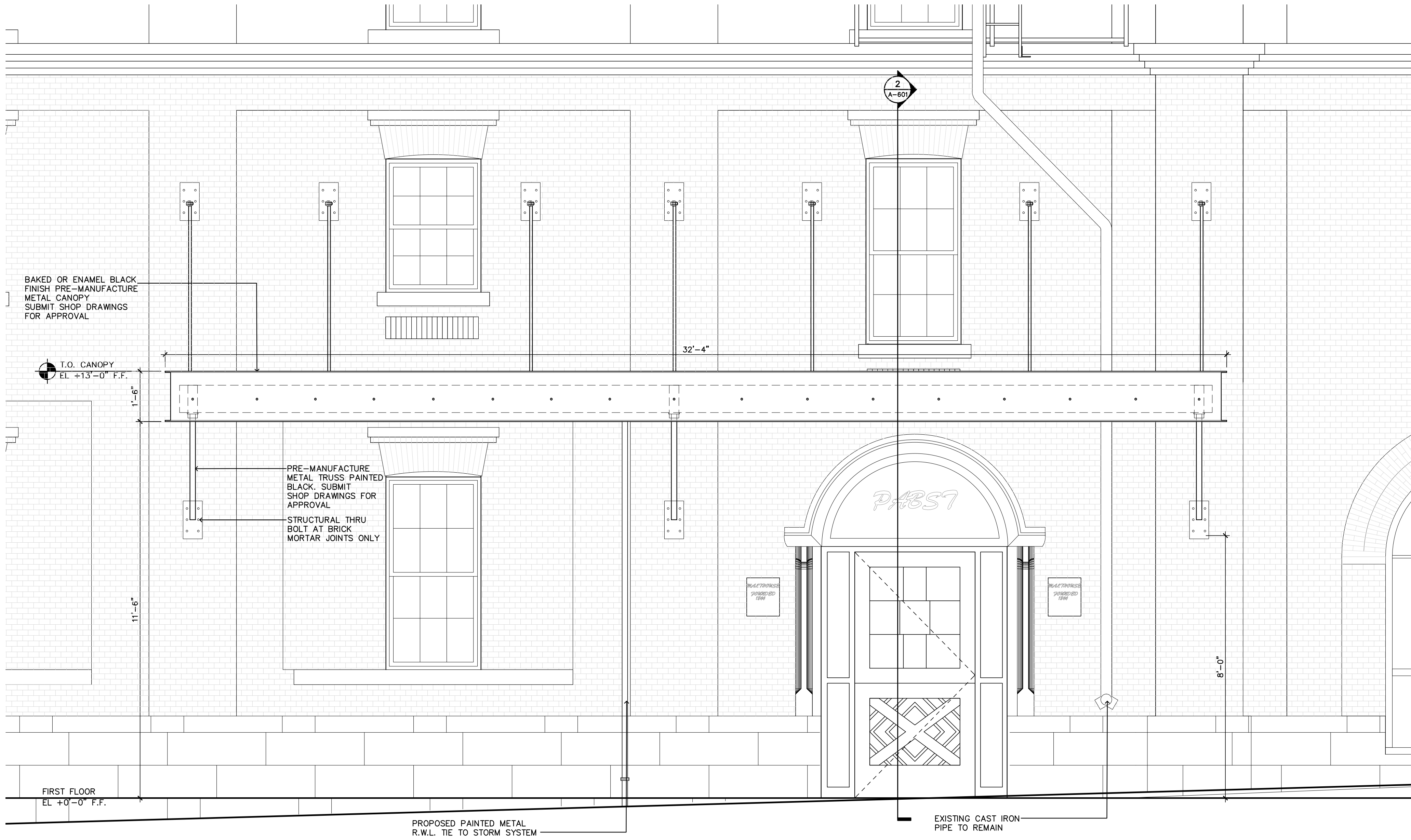
1 PARTIAL BUILDING ELEVATION PROPOSED ENTRANCE CANOPY SCALE: 1/2" = 1'-0"
